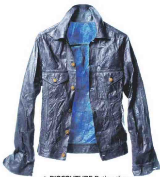
▲ BIOCOUTURE Rather than relying on plant material or petrochemicals, this prototype for a clothing line is based on bacteria in a sugary green-tea solution. After two or three weeks, the bacteria produce a 'skin' on the surface of the liquid that can be dried flat and then cut, sewn and dyed.
